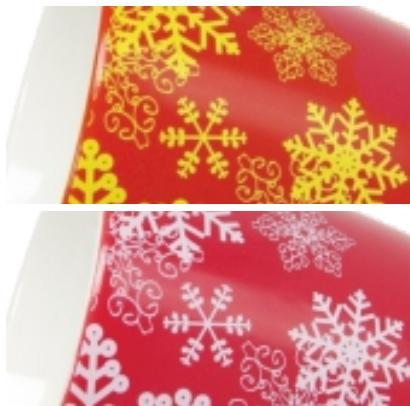
**Ceramic decal** is the main technique for decorating porcelain. This technique consists in printing by using ceramic paints. While firing the decoration on the ceramic melts and builds upon the surface of the product. This creates permanent bond between the decoration and the surface.
